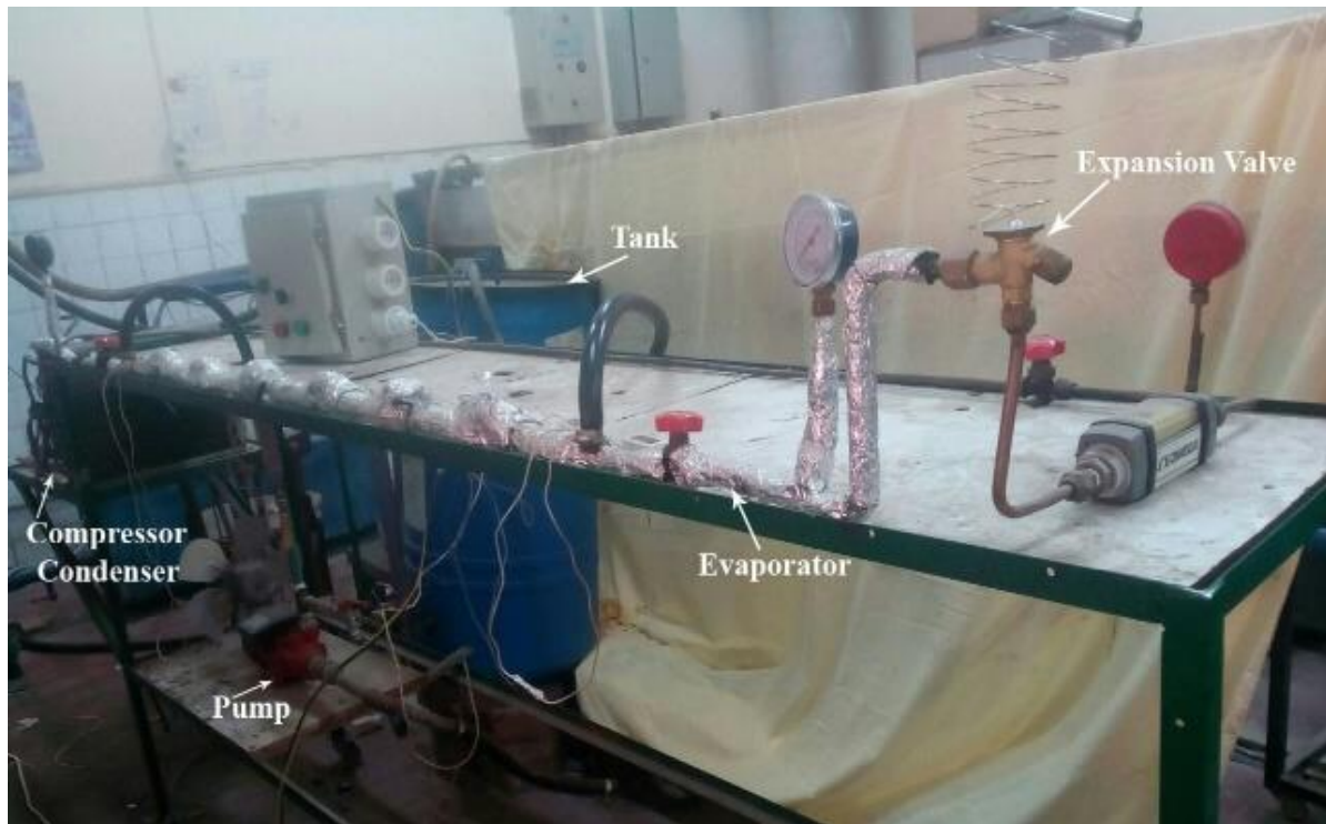
Fig. 2: Photograph of the experimental test rig
